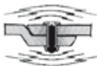
Mandrel locked against falling out
